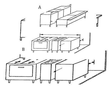
Recommended EQUIPMENT spacing; provided access is available from both ends:
