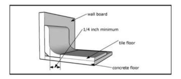
Example of quarry tile cove base flush with floor.
