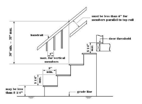
FIGURE 3.11 Stair and Rail Geometry
