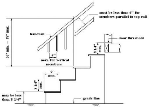
FIGURE 3.11 Stair and Rail Geometry
